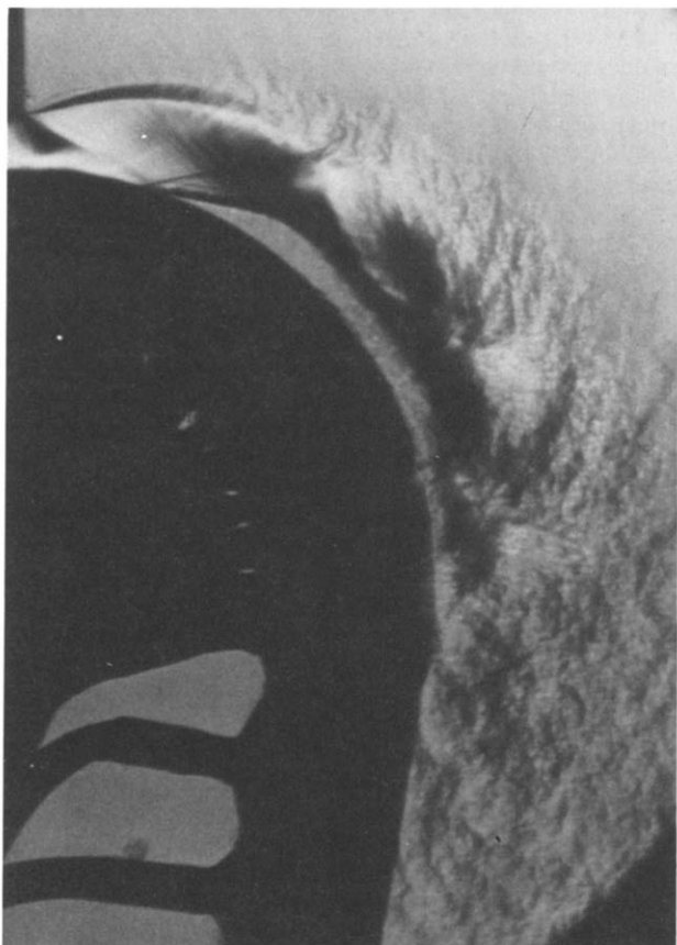
Figure 13 Spark Schlieren, p_a/p_0=0.244 , slot=4 mm, horizontal density gradients
